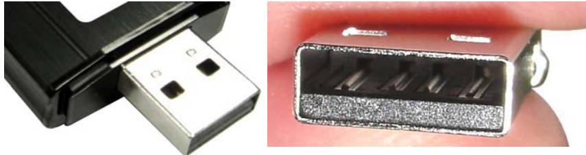
Figure- 4: QDT-2010 USB Flash Disk USB Connector Type A
